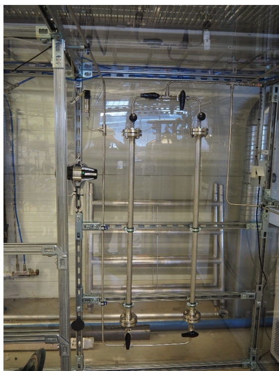
Figure 2-3. The drying system of the CCLU
