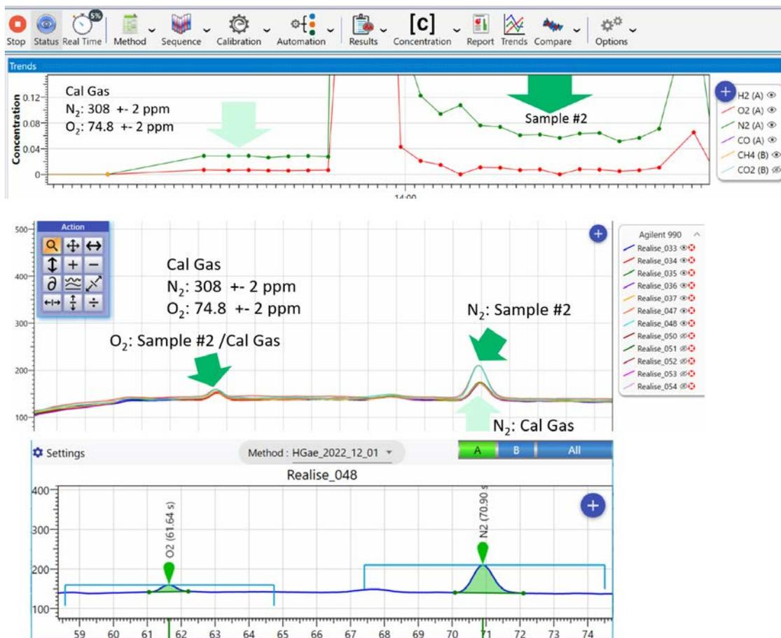
Figure 3-8: Cal gas injection and sample analysis
