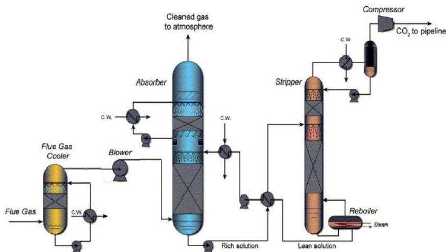
**Figure 2 Overview of the amine process (Dept. Process technology, SINTEF)**
